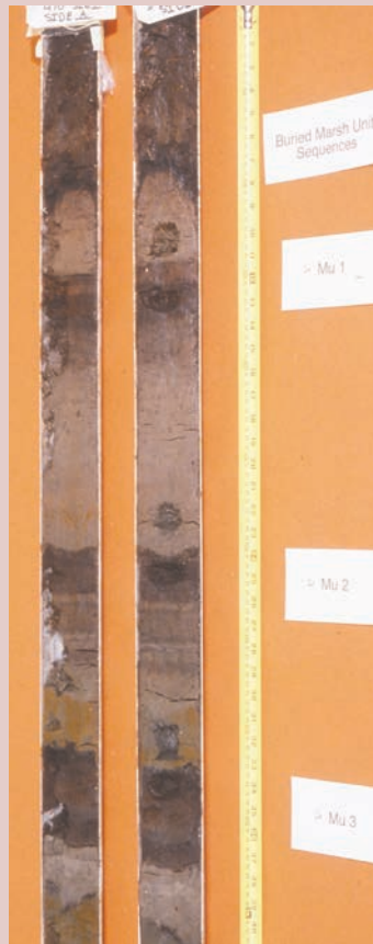
Figure 12. Episodically submerged peat horizons (dark) buried by bay mud (light) from great earthquake subsidence events (mean recurrence interval 400–500 years) in Coos Bay, Oregon. Each burial event represents about 1.0 m of rapid sea-level rise (see Figure 11 for details). Interseismic uplift and sedimentation permit the mudflat to convert back to a marsh, before the next earthquake subsidence (Barnett, 1997).
