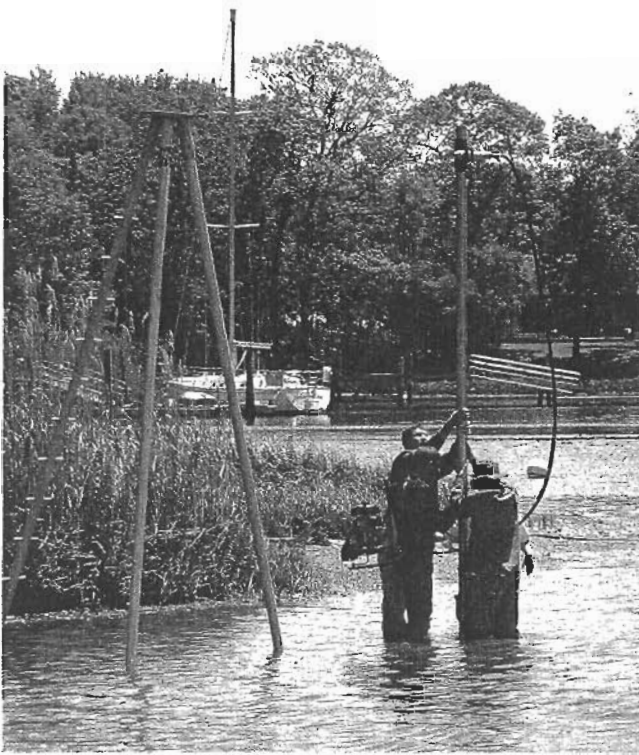
Figure V3 Small, portable vibracore. A backpack power unit operates this pneumatic vibracore; the core barrel is stabilized by hand as the unit penetrates the marsh sediments. The lightweight aluminum A-frame is carried to the site and waits for use in retrieval of the core (photo courtesy of Steve Krupa, South Florida Water Management District, West Palm Beach, Florida).
